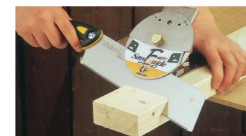
VERTICAL 45°-90° By adjusting the vertical angle bracket, cuts up to 45° forward or backward can be performed.
