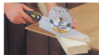
PARALLEL 45°-90° By adjusting the parallel angle bracket, cuts from 45° to the right or left can be performed.
